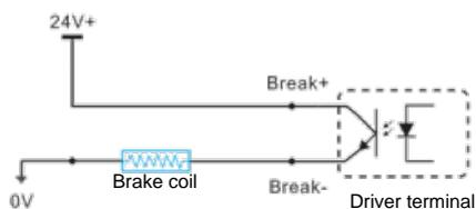
Break is the brake control signal, which is set by software. Do not connect the brake coil reversely (red+, black-).
